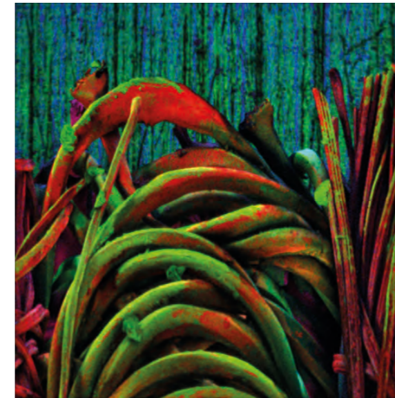
Overlay: C 4 H 9 + (red), Na + (green), Al + (blue) Primary ion: Bi 3 + , Field of view: 500 x 500 μm 2 , Pixel size: 1 μm
